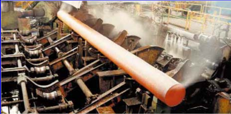
Pipe coming out of the expander
