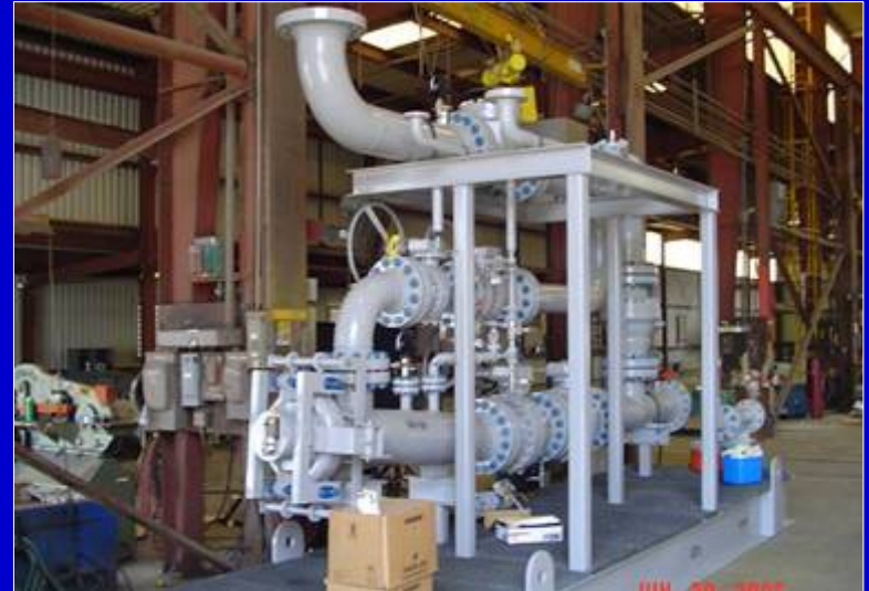
Pig Launcher Skid Fabrication
