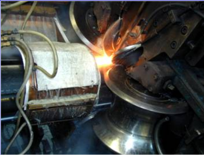
Induction welding - CORUS
