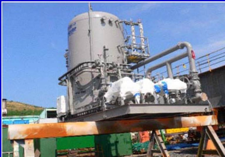
Gas Flotation Skid
